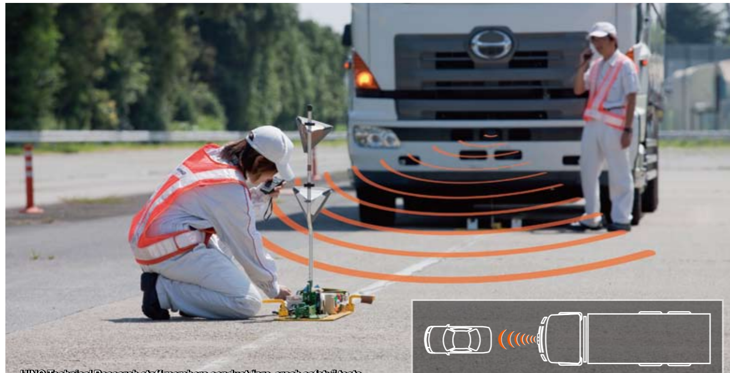
HINO Technical Research staff members conduct "pre-crash safety" tests
