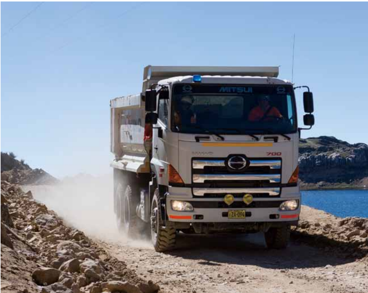
The trucks get their power from additional turbos that have been outfitted for highland areas where oxygen concentration is low.
