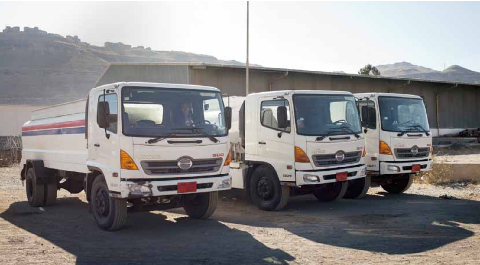
These HINO500 Series trucks have been fitted for petroleum transport.
